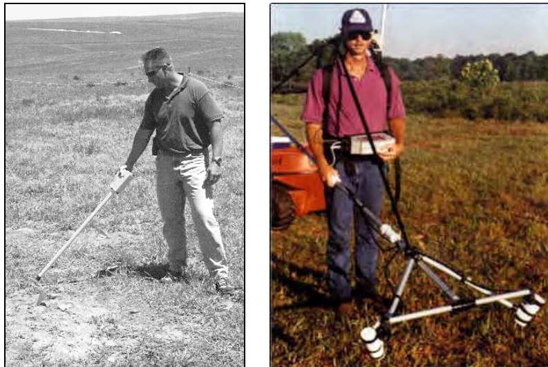
Figure 3-11. Schonstedt used in mag-and-flag operation (left) and G858 used in a hand-held mapping operation (right) (Photograph courtesy of Geometrics).
