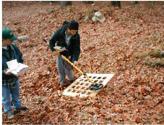
Figure 7-2. Cued identification of anomalies using an EM-61HH and template.
