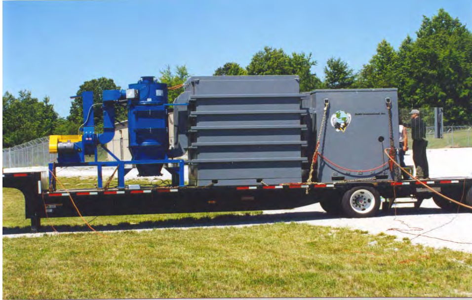
Figure 10-3. T-10 mobile detonation chamber. (Photo courtesy of DeMil International.)
