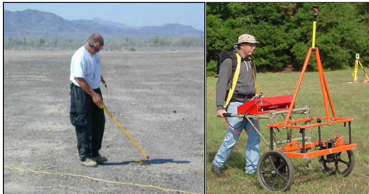
Figure 3-1. Schonstedt magnetometer (left) and Geonics EM61-MK2 EMI (right).
