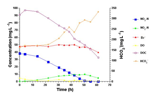
Figure 7-8. Concentration vs. Time for Selected Analytes Involved in or Affected by Microbial Denitrification Following Injection in a Microcosm Amended with 100 mg C L<sup>-1</sup>
