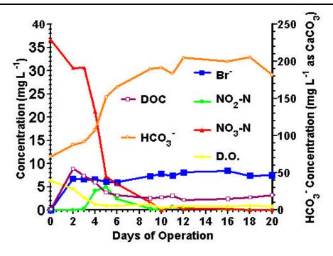
Figure 7-11. Anion, D.O.C. and D.O. Concentration in Inner Well #3. Complete Reduction Occurs in the Observation Wells Located in the Impacted Zones.
