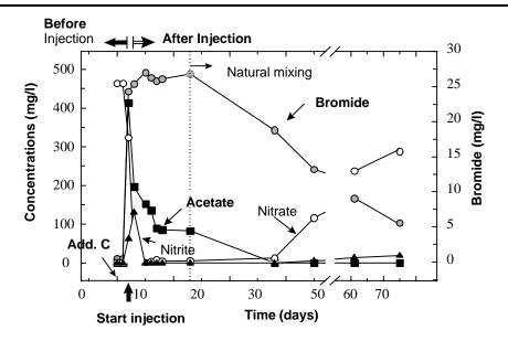
Figure 7-3. Reaction Concentration Curves Measured During an *In Situ* Biodenitrification Test
