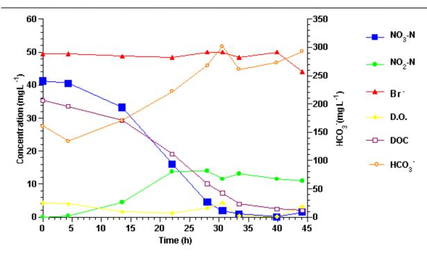
Figure 7-7. Concentration vs. Time for Selected Analytes Involved in or Affected by Microbial Denitrification in a Microcosm Amended with 50-mg C L<sup>-1</sup>
