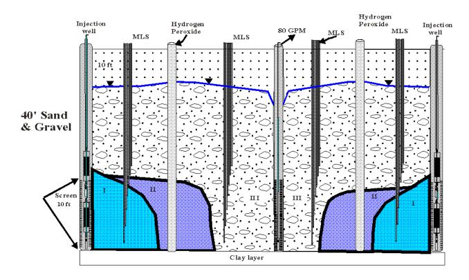
Figure 7-10. Vertical Section of Daisy Injection System. (I Reducing Zone, II Oxidizing Zone, III Treated Water Zone)
