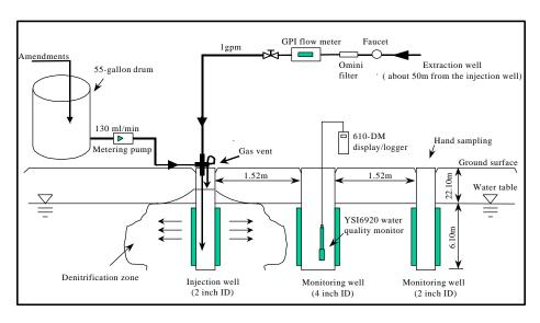
Figure 7-4. Modified Schematic Diagram of Continuous Denitrification Field Ttest
