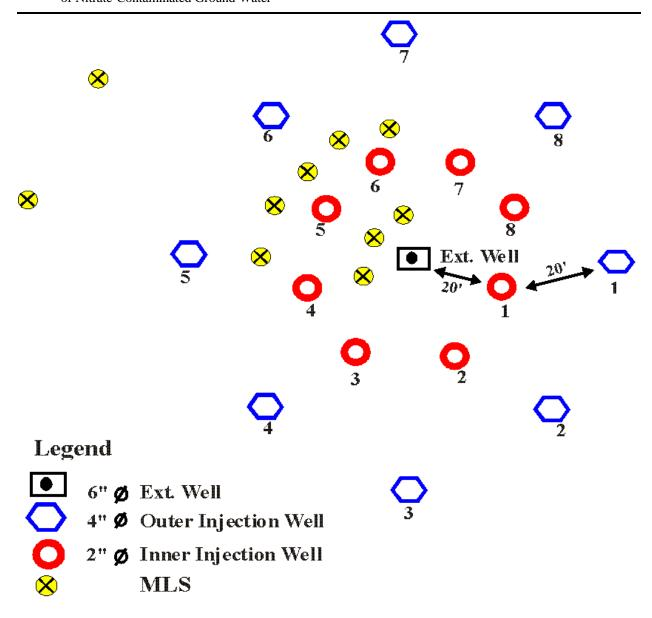
Figure 7-9. Layout of Daisy Injection System
