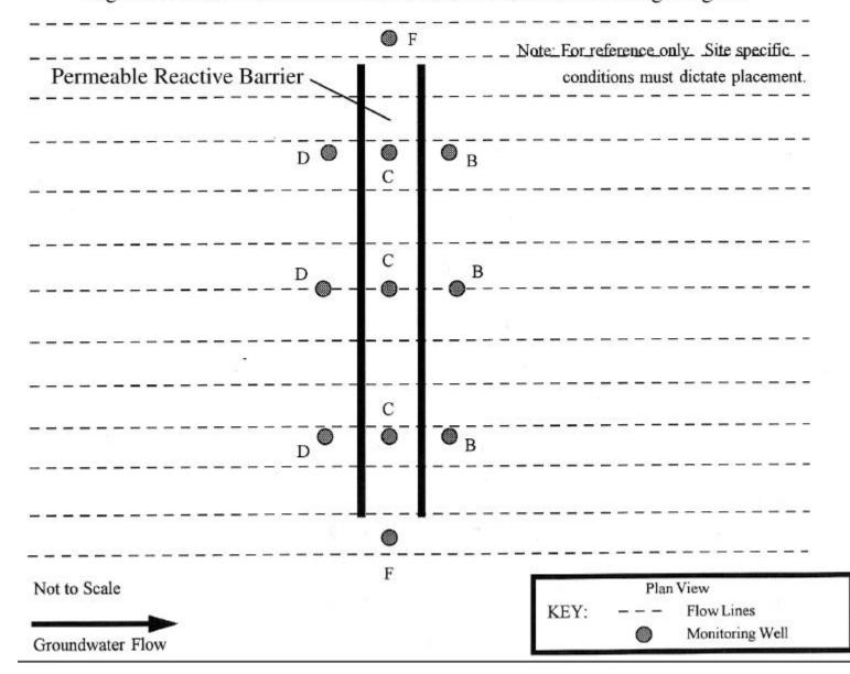
Figure 6-2 Continuous Permeable Reactive Barrier Monitoring Diagram
