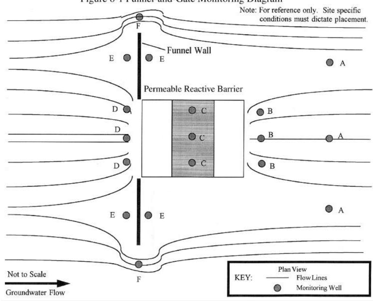
Figure 6-1 Funnel-and-Gate Monitoring Diagram
