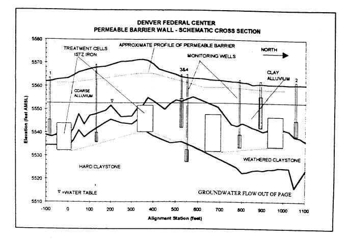
The diagram above conceptually illustrates in cross section, the groundwater monitoring system for the Denver Federal Center (DFC) funnel-and-gate system. The aquifer at DFC consists of three lithologic units of decreasing permeability with depth: alluvium, weathered claystone, and hard claystone.
