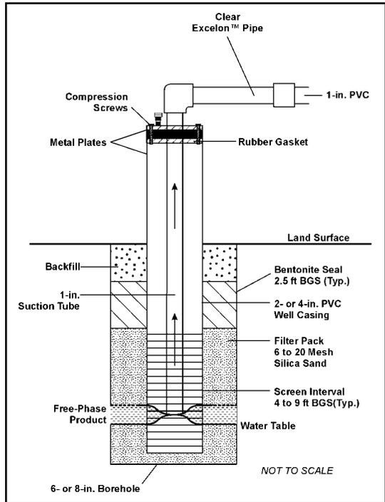
Figure 3. Diagram of Extraction Well
