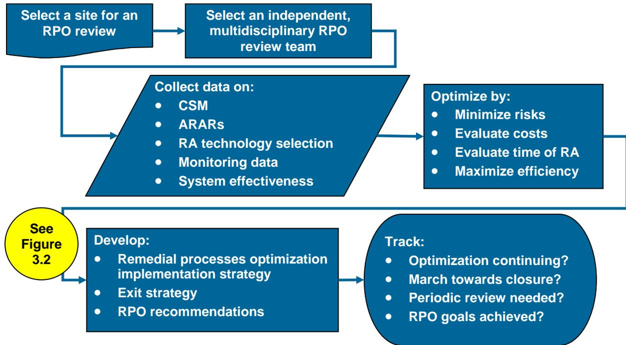
Figure 3-1. Overview of conducting an RPO evaluation.
