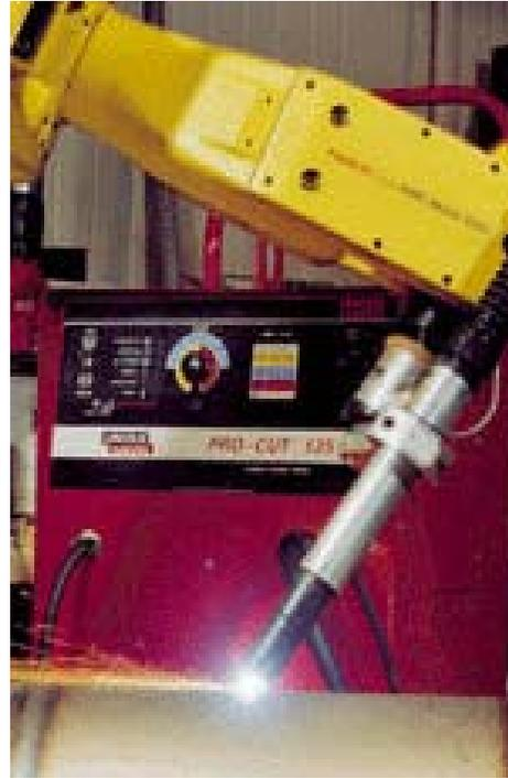
**Figure 6-4. Plasma-arc cutting torch.**
