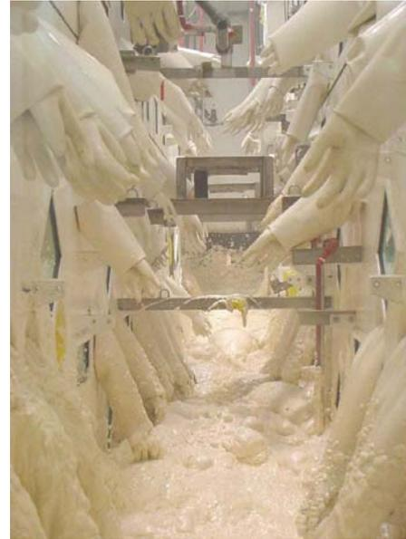
**Figure 6-12. Glovebox filling with structural foam.**
