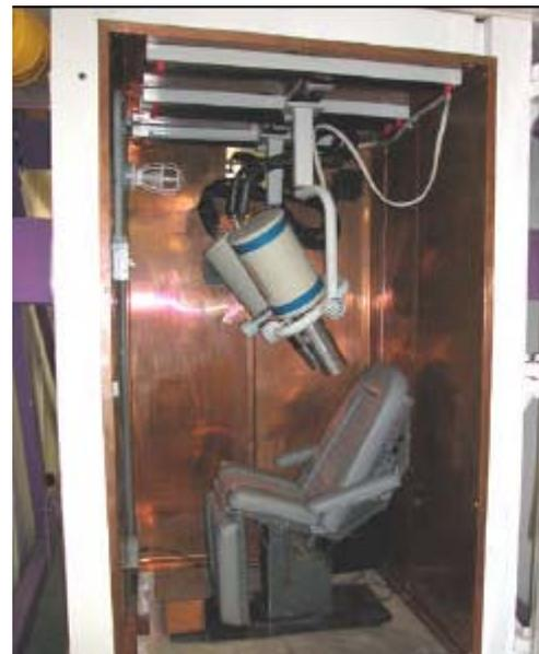
**Figure 6-14. View of the shielded room and counter.**
