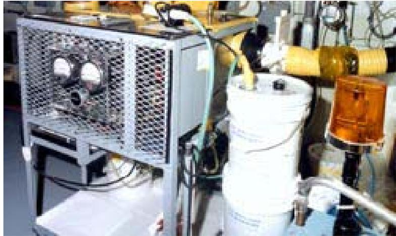
**Figure 6-3. Use of the aerosol fogging equipment is intended to downgrade the personal protective equipment requirements for room entry from supplied-air suits to standard powered air-purifying respirators.**
