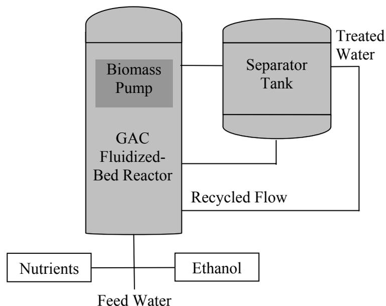
**Figure 6-5. General schematic of a fluidized bed reactor.**
