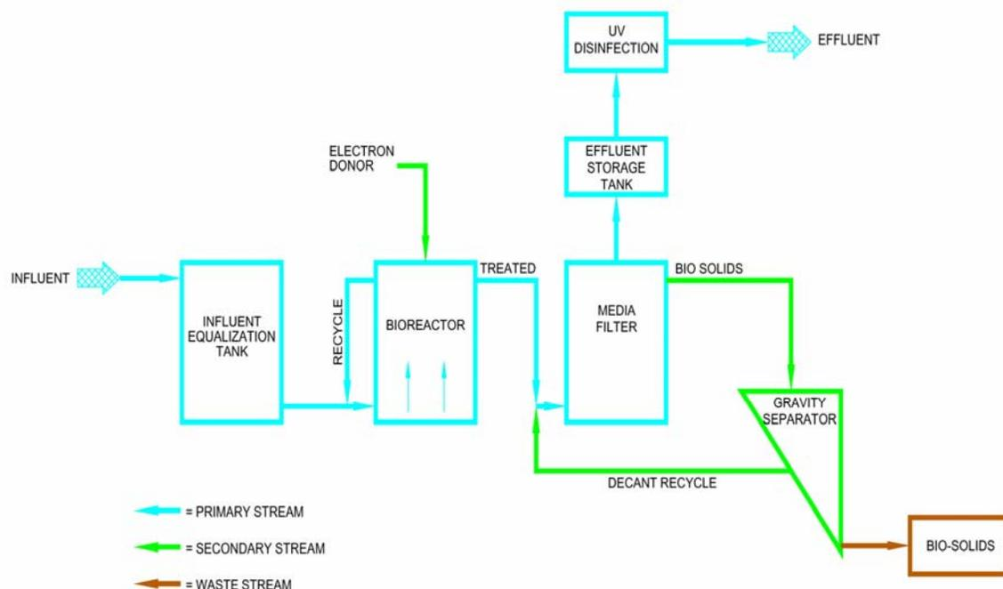
**Figure 6-3. General schematic of ex situ bioremediation.**
