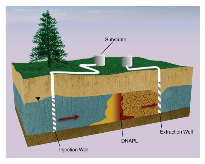
Figure 4-2. Schematic for ISB applications for source containment
