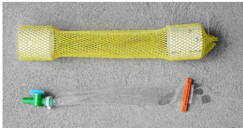
Figure 5-3. Partially assembled dialysis sampler before filling with deionized water with external supports installed in the protective mesh. (~2.5 inches in diameter by 24 inches long)
