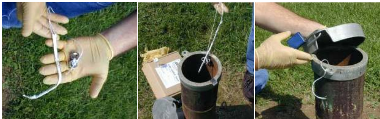
Figure 2-5. GORE Module deployment. L to R: Module and weights secured to string, lowering module into well, and capping well after installation. Note: String is secured to wellhead before lowering module into well.
