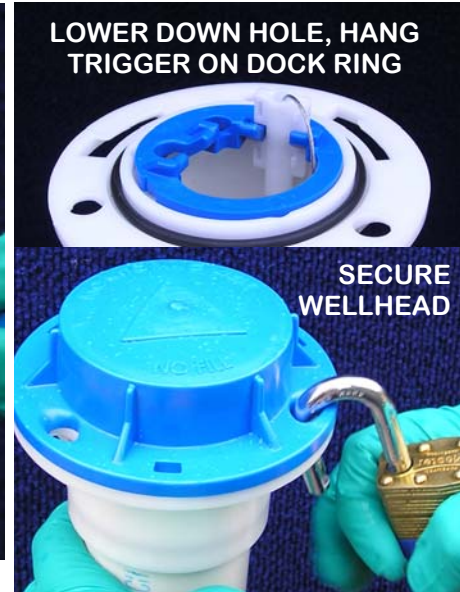
Figure 4-7. Securing sampler into wellhead docking station.
