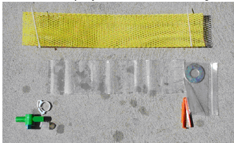
Figure 5-2. Parts of a dialysis sampler before assembly. (~2.5 inches in diameter by 24 inches long)
