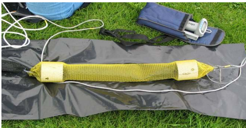
Figure 5-1. Regenerated-cellulose dialysis membrane sampler. (2.5 inches in diameter by 24 inches long)
