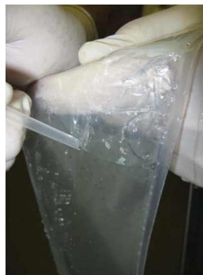
Figure 3-10. HydraSleeve flexible reed valve.
