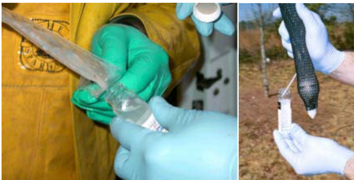
Figure 8-6. Transferring sample to VOA vials. Discharge of PDB sampler using a discharge straw in the right photo.
