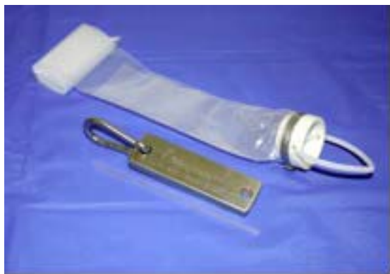
Figure 2-1. 1.5-inch HydraSleeve™ and stainless steel weight (1-liter capacity)
