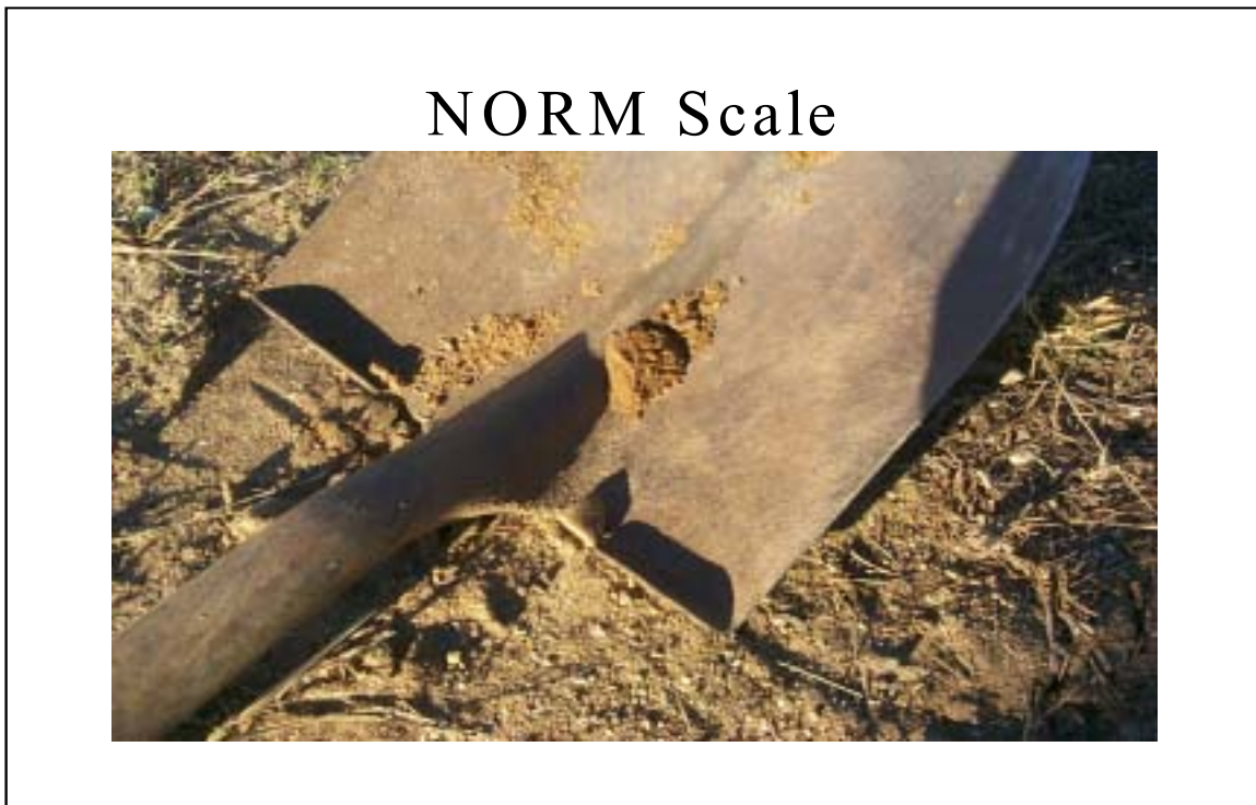
Figure G-6. NORM pipe scale on a shovel
