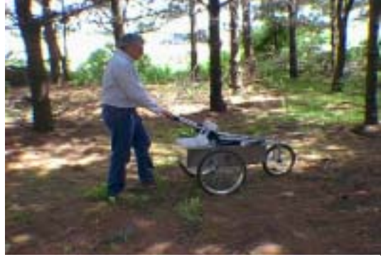
Figure 2-3. Radiation scanning system
