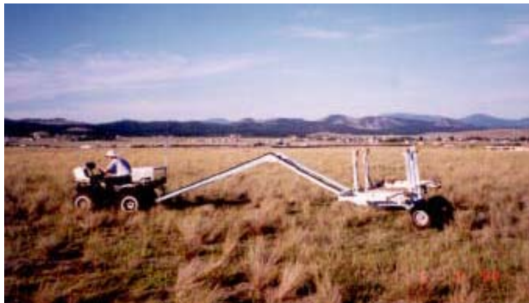
Figure 4-3. Multiple-sensor, towed-array system.
