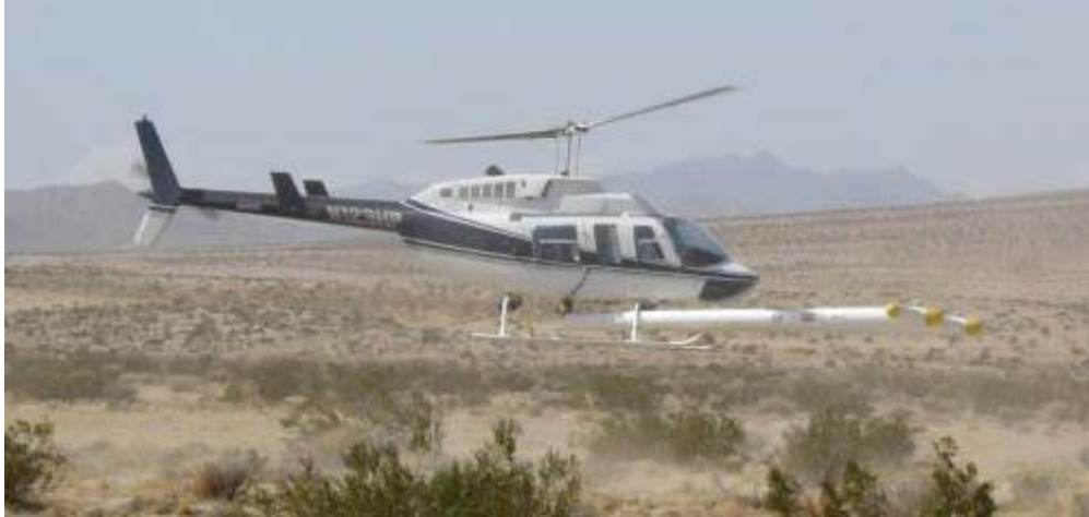
Figure 2-4. A helicopter-deployed magnetometer array during a geophysical survey.
