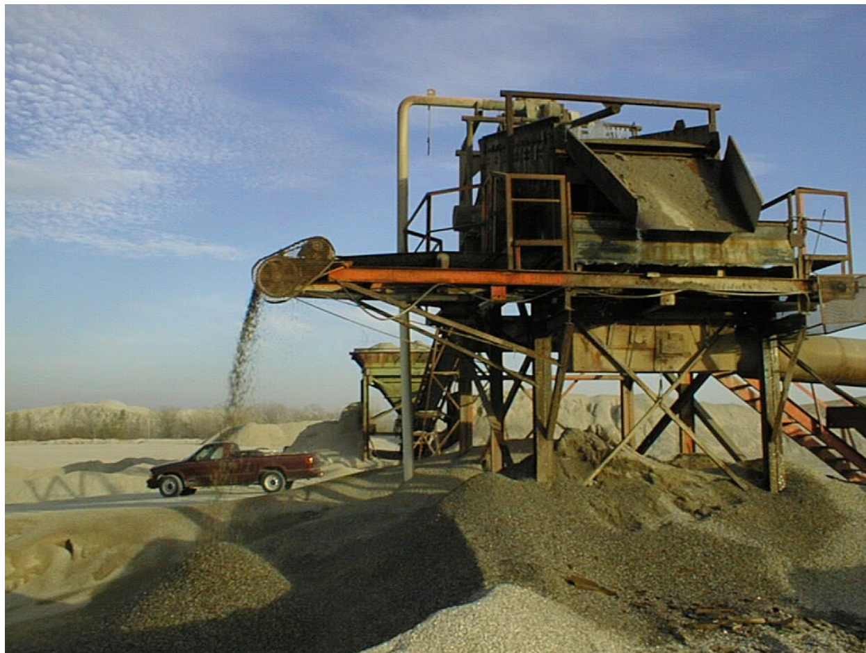
Figure 4-3. Wet screening (washing) of chat to separate different size fractions and remove fines.
