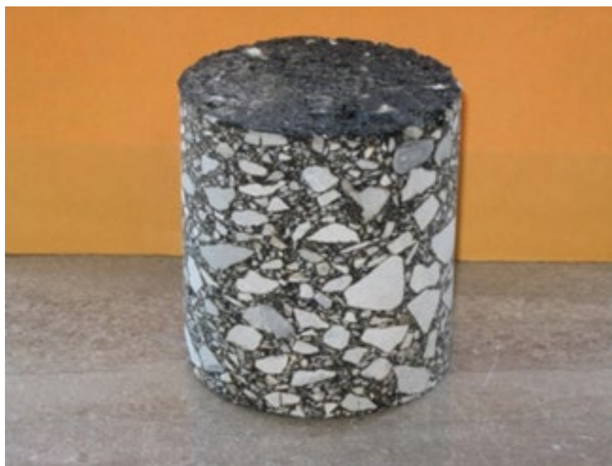
Figure 4-1. Test Specimen of asphalt concrete with mining waste (chat) making up part of the aggregate mix.
