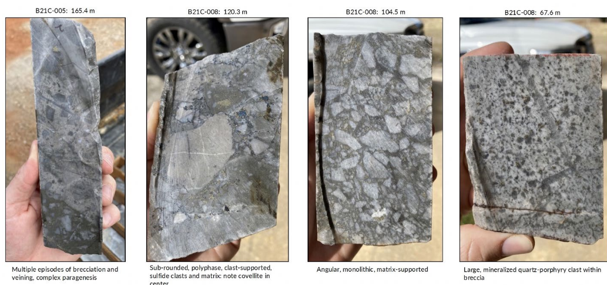
Figure 6-25. Core drilled from the Brewer Site demonstrating differences in alteration.
