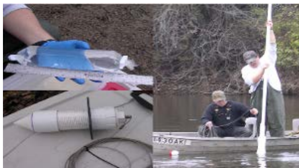
Peeper sampler (l), sampler installation (r).
