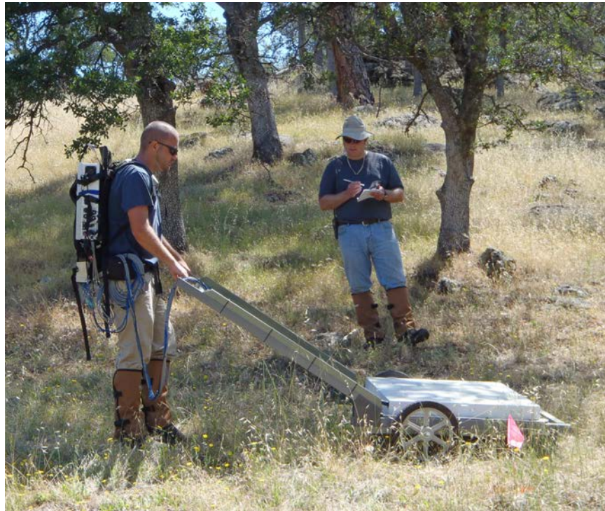
Figure A-1. Treed area at the former Camp Beale demonstration site required the use of man-portable systems to conduct classification surveys.
