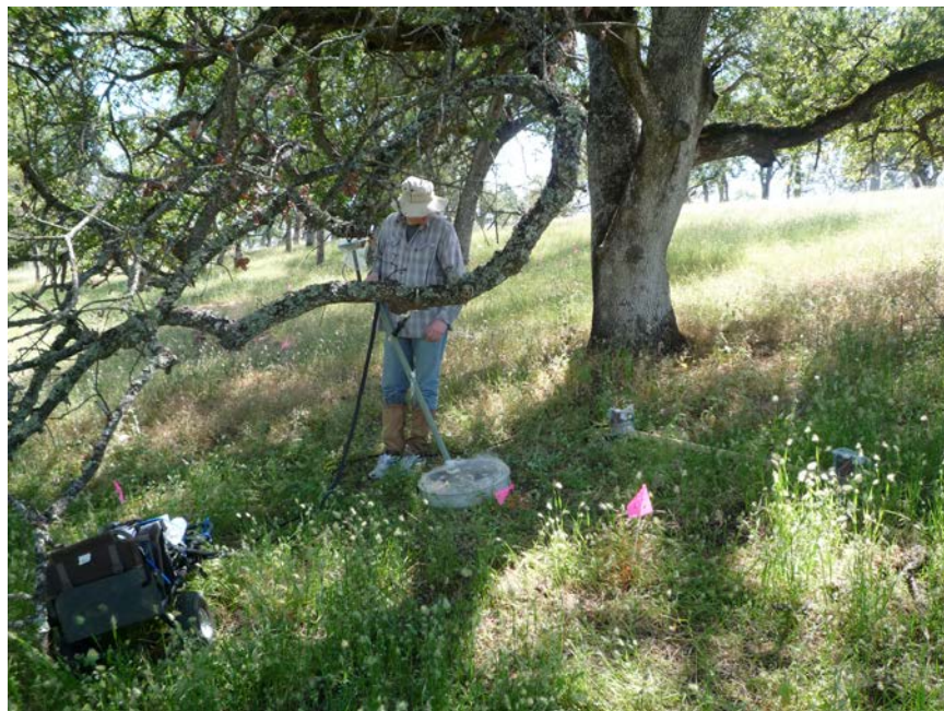
Figure A-2. Treed areas can obstruct the acquisition of GPS satellite signals.
