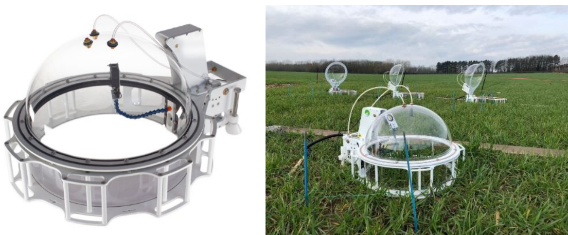
Figure 1. Photographs of mass-flux chambers.
