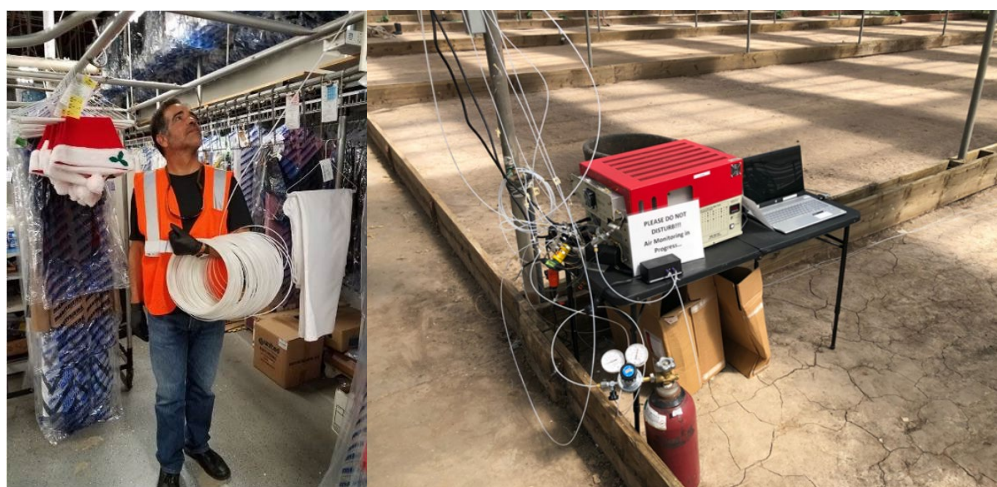
Figure 2. Automated gas chromatography sample tubing deployment (left) and the monitoring system in the field with tubing connected to stream selector valve sample inlets (right). Note that each tubing run is labeled and assigned a valve port so that each analytical result is associated with a specific monitoring location.
