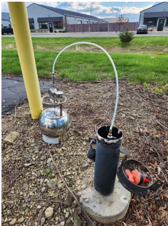
Figure 6. Soil vapor sampling from an existing groundwater monitoring well.
