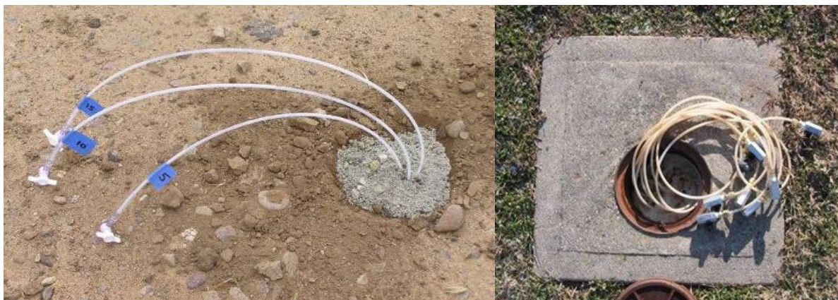
Figure 4. Examples of typical multi-nested soil vapor probes.
