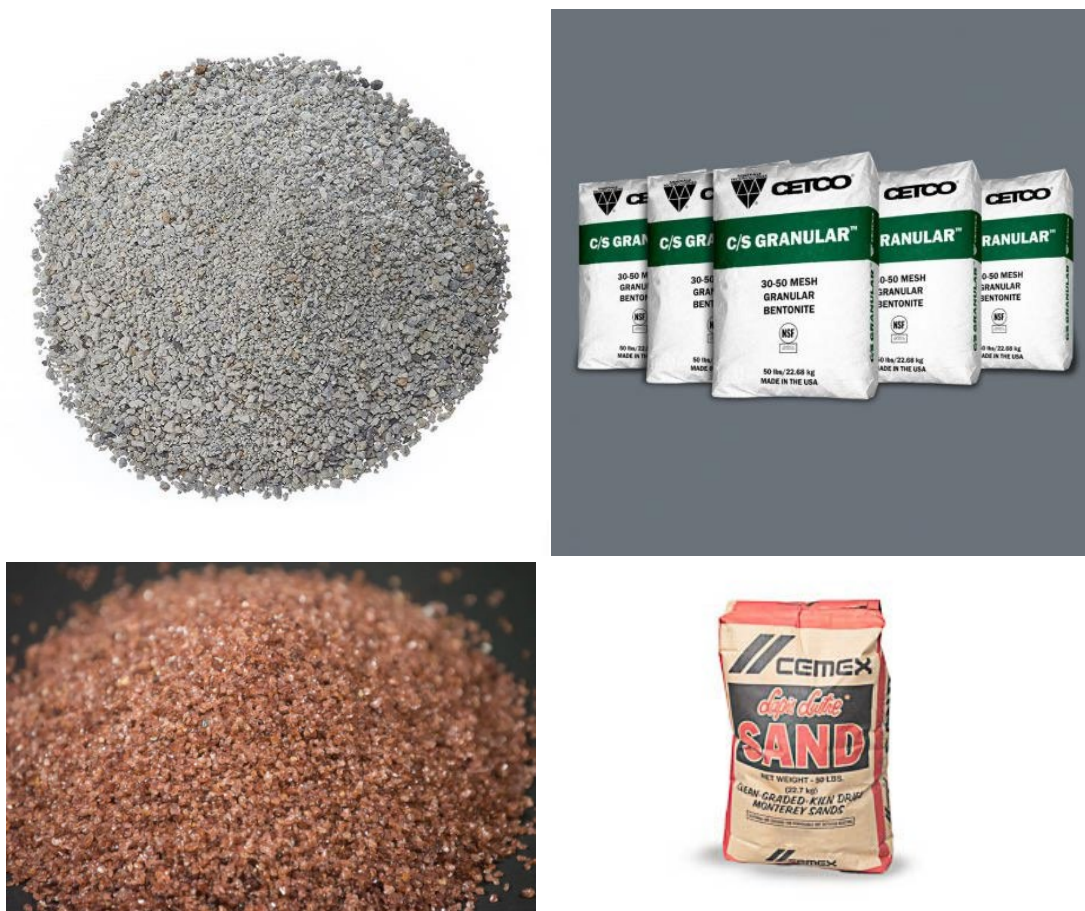
Figure 9. Photographs of typical granular bentonite (top) and sand (bottom) used during the soil vapor probe installation process.
