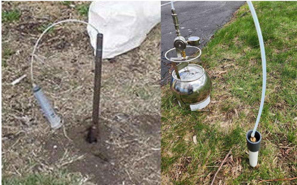
Figure 1. Photographs of driven soil vapor probes. Note the probe on the left has no seal.
