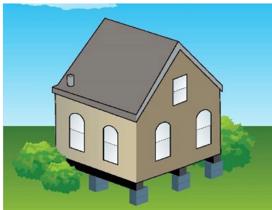
Figure 2. Schematic of a block-and-beam foundation.
