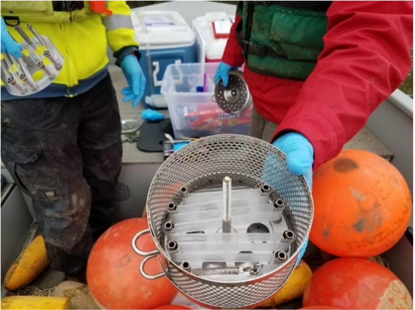
Figure 5-36. SPMD carrier assembly inside the protective canister. Source: Anchor QEA, used with permission.
