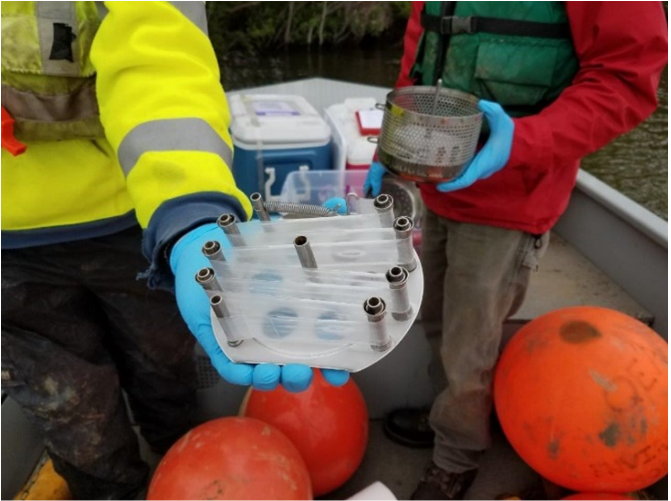
Figure 5-35. SPMD carrier assembly and triolein film. Source: Anchor QEA, used with permission.
