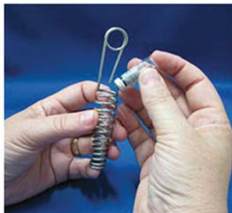
Aligning WMS™ sampler in wire hanger
