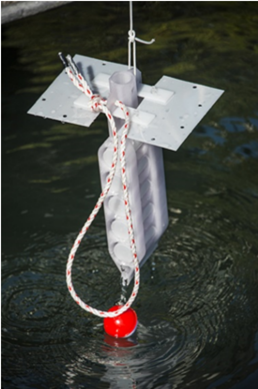
Figure 5-18. SPeeper modified bottle peepers are designed for diverless deployment in sediments. Source: SIREM, used with permission.
