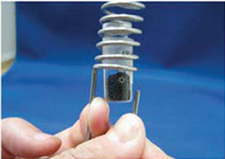
Removing WMS™ sampler from wire hanger
