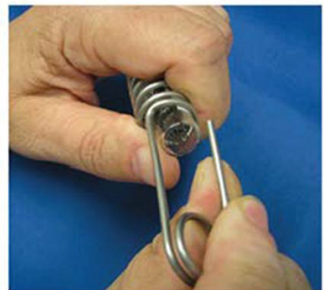
Bending wire to insert WMS™ sampler
