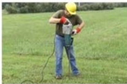
Rotary hammer drill and 36 in (1 m) long, 0.5 in (1 cm) diameter carbide-tipped bit
