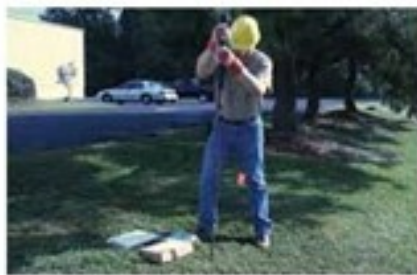
Slide hammer and tile probe
