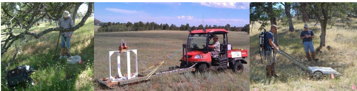
Figure 4. Advanced EMI sensors include hand-held (left), sled-mounted (middle), and cart-mounted (right) units.
